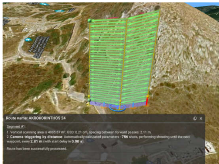
Figure 3. Scheduled flight with calculated data, flight time, number of photos, GSD, and area covered
