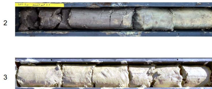
Figure 2. Former marsh: peaty facies at the top left and clayey facies in the rest of the cores (S26).
