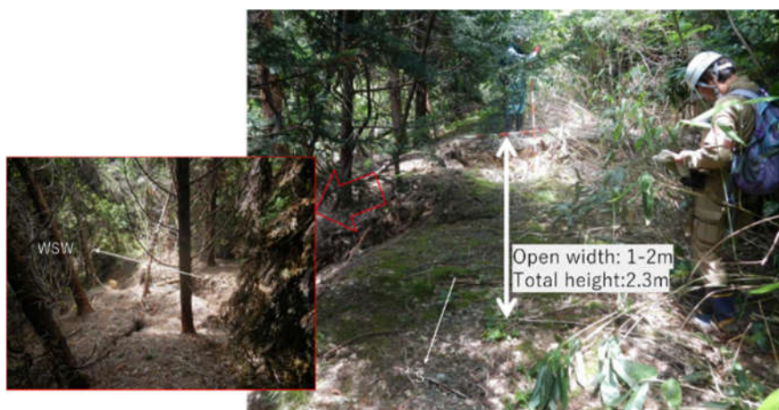
Figure 10. Image at Loc. IV. Step-fault like deformation of north side of depression and scarps extending to WNW direction
