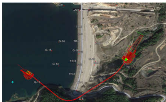
Figure 2. General layout of the diversion tunnel of the Triantafyllia dam (in red). In dots the sampling boreholes.
