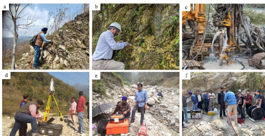
Figure 4. Showing Photographs of Confirmatory Surface Geological and Geophysical studies. (a) Geological survey along HRT alignment. (b) Assessing rock strength using Schmidt Hammer. (c) Drilling activity (d) Topographical survey (e) Resistivity Imaging. (f) Cross hole P-wave Tomography.
