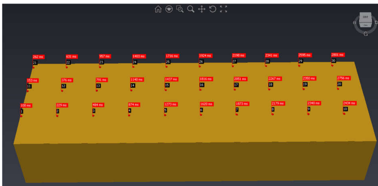
Figure 6. Delays applied to the holes using Seisblast Promax software
