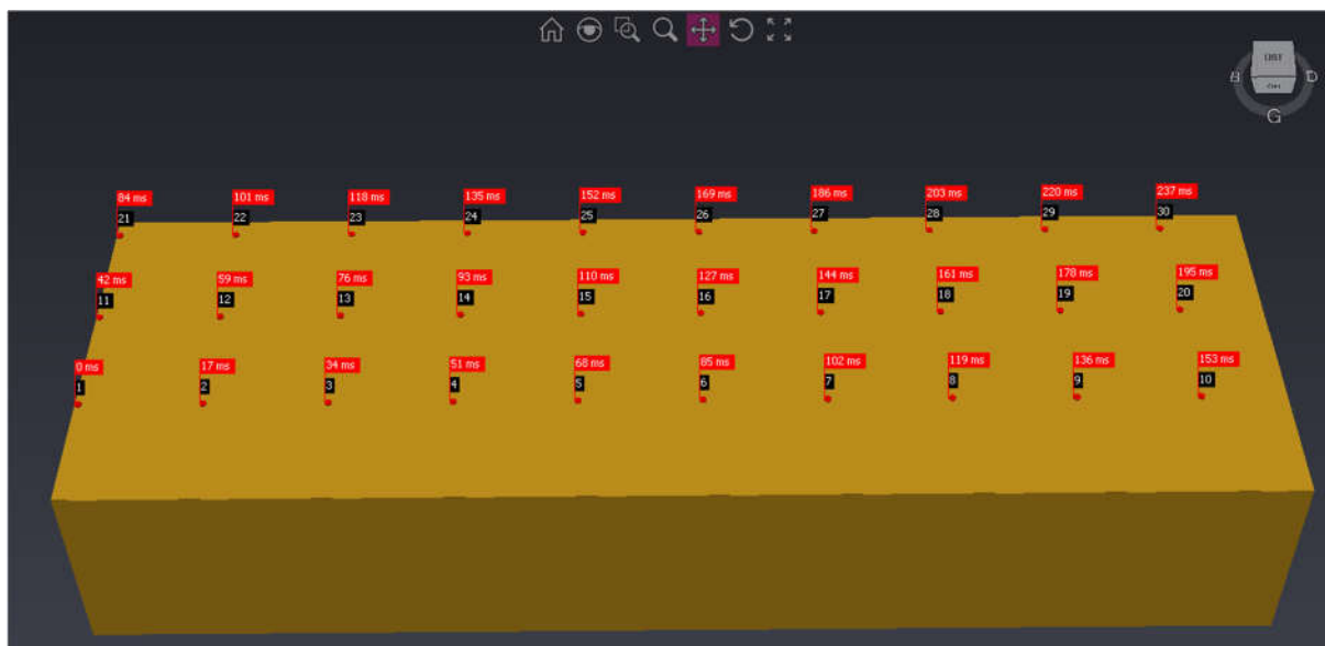
Figure 5. Delays applied to the holes for conventional blasting system
